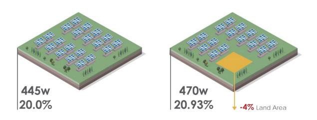
Using tiger module can save 4% land area comparing with 445w module.
