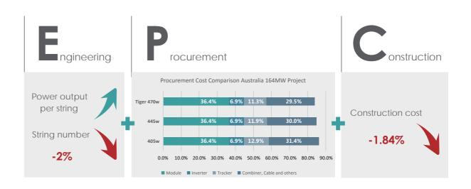
Comparing with 445w, using tiger module can save >1.2% EPC cost.
