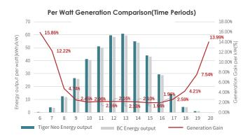
**3.Distinct "Early Start and Late Shutdown" Characteristics:** At 6 AM, the power generation per-watt of JinkoSolar Tiger Neo modules achieved a gain of **15.86%** compared to N-type BC modules, entering the effective power generation state earlier; at 8 PM, the gain reached **13.99%**, effectively extending the daily power generation duration.
